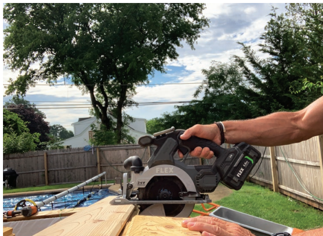
The Flex 6 1/2-inch cordless saw has a blade-left design, an adjustable dust port, and a cutting capacity of 2 9/16 inches.
