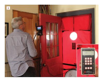
The author switched from using his old workhorse DG-700 model (inset photo) to a DG-1000 (1), though he still uses the DG-700 for tests requiring multiple blower doors.
