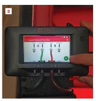
Large pictographs help users set up the manometer for testing. Here, the home screen shows the unit's five primary apps (2). Tests can be launched from either the gauge app or the tubing assistance app. Tubing assistance shows the user which pressure taps to hook the diagnostic tubing to, depending on the airflow-measuring task (3). The green arrow button is the "launch with current configuration" button, which takes the user to the gauge app.
