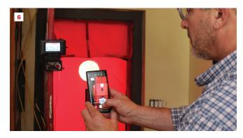
Label: Oct 9, 2021 3:39:07 PM Ch A Value: -49.8 Pa (adj) Baseline: -0.1 Pa Ch B Value: 2028 Ch B Mode: Flow@50 (cfm) Ch B Flow Units: cfm Ch B Pressure: -127.6 Pa Flow Device: Model 3 Fan Flow Device Config: Ring A Time Average: 5 Second Area: 0.0 ft<sup>2</sup> Volume: 0.0 ft<sup>3</sup> Timestamp: Oct 9, 2021 3:39:07 PM Gauge Serial Number: DG1000-5661 Gauge Calibration Date: May 1, 2020 Comment: Smith res
