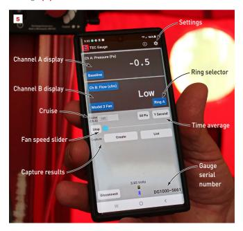
The most substantial upgrade of the DG-1000 over the DG-700 is its connectivity to smartphones and tablets. TEC's gauge app allows users to operate the DG-1000 remotely and find, say, a leaky spot in the attic. Here, the gauge app screen appears on the author's smartphone (5). Once activated, the phone app overrides the unit's controls.
