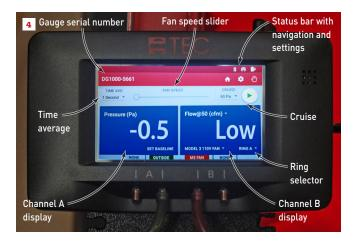
In addition to familiar channel A and channel B displays, the gauge app screen contains functions such as fan speed, time average, and cruise, which automatically starts the blower door fan running to achieve, in this case, ACH50. The unit's serial number is displayed in the upper left-hand corner, which is useful during calls for tech support or maintenance. The status bar contains navigation and settings (4).
