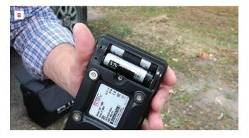
The DG-1000 uses two lithium-ion rechargeable batteries with a 15-hour runtime (depending on WiFi use and screen brightness). Four strong neodymium magnets (shown here below the batteries) hold the unit to the metal gauge board (8).
