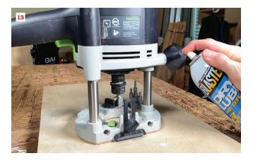
For cutting mortises for door hinges, the author uses a simple plywood template that he fastens to the workpiece with double-sided tape (11). The template is sized to fit the hinge template router bit, which typically has a short cutter-to-bearing distance since most hinges aren't very deep (12). An occasional spray with a dry lubricant will prevent the tubes on a plunge router from gathering sawdust and sticking (13).
