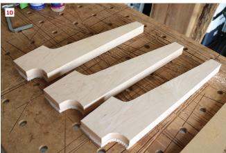
To make duplicate table-top supports, the author first makes a pattern, using it to trace the support's outline on the workpiece, which he cuts out with a band saw. Then he uses double-sided tape to attach the pattern to the workpiece and finishes cutting it out with a flush trim bit with a top-mount bearing (9). After making the initial cut, the pattern can be removed from the stock and the cut can be completed using the same flush trim bit (10).
