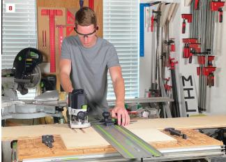
Before cutting an edge profile with a router bit fitted with a bottom-mount bearing, the author sands the edge of the workpiece to ensure that the bearing has a smooth surface to follow (7). To ensure a snug fit when cutting dados in shelf supports, the author uses an slightly undersized straight cut router bit and guides the router with a Festool guide stop and track (8).
