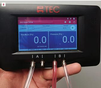
During a ZPD test of attic pressure with respect to the living space, a manometer that shows this zone at a pressure near 50 pascals (1) indicates that the ceiling air barrier is nearly perfect, because the attic is at the same pressure as the outside. However, if the zone pressure reads near zero (2), the attic zone is completely connected to both outside and inside.
