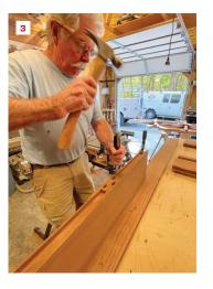
The author typically builds standard 13/4inch doors on site with a Festool Domino XL joiner and OF 1400 router set up with a double fence (1). The new, oversized, 21/4-inch doors were built in the shop using the same tools and techniques (2). Here, three mortises are cut in a staggered pattern rather than in line to strengthen each side of the thick door (3).
