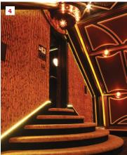
The entry stairs to a home cinema the author was commissioned to design and build are elliptical. After developing them in CAD (3), he broke the stairs into components that fit into 4-by-8-foot rectangles. Each of those files were saved separately and loaded into the CNC machine, then cut out of shop-grade birch plywood. The parts were assembled in a few hours on site. The completed stairs were wrapped in carpet (4).
