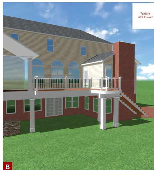
Figure 2. The author uses information from the client worksheet and his library of standard details to create plan views (A) and 3D renderings (B) in Realtime Landscaping Architect CAD software. He then loads the deck's square footage and component list into Projul construction management software, which he has preloaded with pricing, to determine a project's estimated cost and share it with a client in the proposal (C).
