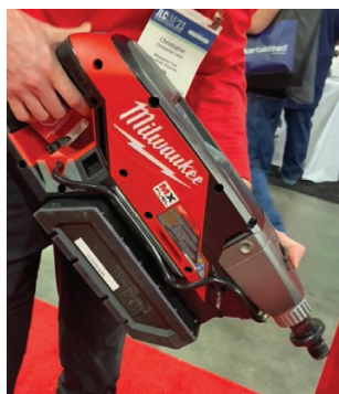
Milwaukee's MX Fuel core drill can be hand-held (left) or mounted in a drill stand for holes larger than 3 inches (right).
