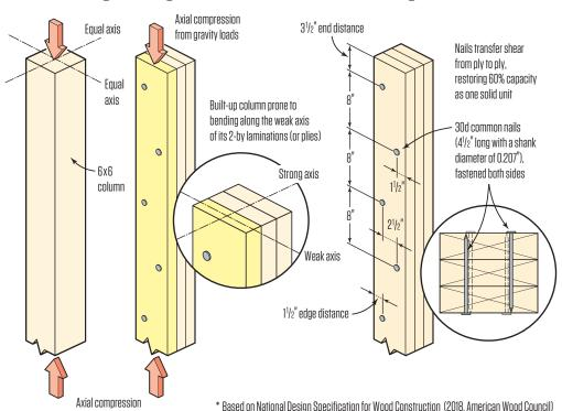
Axial loads on a builtup column tend to act on the weak axis of each member, rather than on the whole assembly as they would with a solidsawn column (far left). Even when the plies are fastened together per NDS specifications (left), the bending strength of a post assembled from three 2x6s is about 60% that of a solid-sawn 6x6 post.
