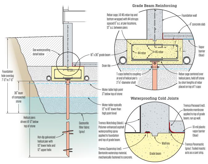
Roof and floor loads are transferred down through the walls to the concrete foundation and steel-reinforced grade-beam footing, which in turn bears on helical piers, each capable of supporting at least 15,000 pounds. Groundwater can move freely through the compacted stone base, while the waterproofing details shown above keep it from entering the crawlspace.
