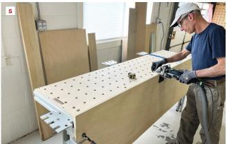
Crosscuts as wide as 24 <sup>3</sup>/4 inches are possible when the guide-rail brackets are fitted to a track saw's guide rail (3). Adding the system's Outriggers to the workbench provides additional support for ripping sheet goods (4). Doors or panels can be clamped vertically to the side of the bench with the addition of optional supports (5).
