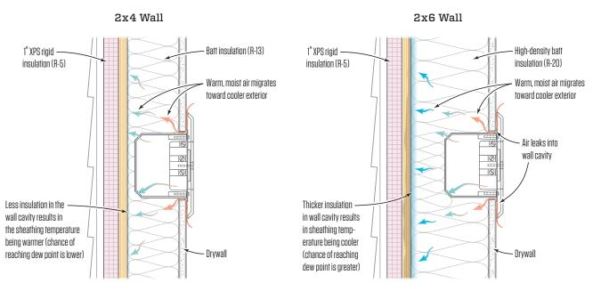
Condensation is more likely to form in the 2x6 wall (right) because, under the same temperature and humidity conditions, the thicker cavity insulation will keep the inside face of the sheathing cooler than will the thinner insulation on the 2x4 wall (left).
