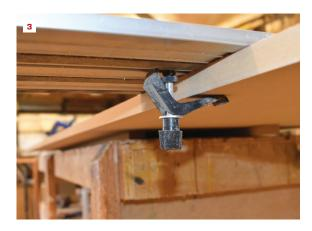
The Kreg ACS plunge saw has a  $6^{1/2}$ -inch-diameter blade and works with the company's 62-inch guide track (1). The saw features a blade-left design (2). Tracks can be joined together with special connectors and fitted with clamps (3).
