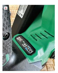
Metabo HPT's 18-gauge brad nailer (4) and 23-gauge pinner (5) both have onboard battery gauges (6), though the company's new 2.0-Ah battery has a simple meter that is easier to read. If a nailer loses power, a reduction valve set (Hitachi 371208 J-394) is available for refilling the air chamber (7).
