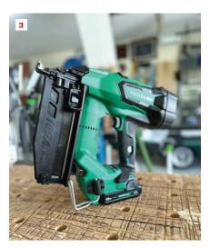
For trim work that requires holding power, the author prefers Metabo HPT's MultiVolt 15-gauge angled finish nailer (1, 2). Metabo HPT's 16-gauge straight finish nailer weighs about a pound less and leaves a smaller hole (3).
