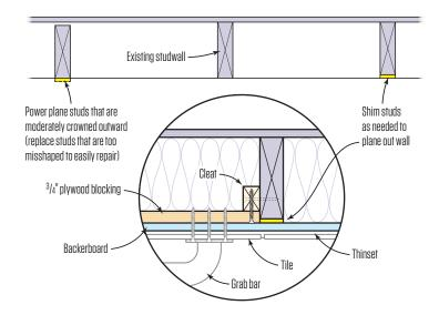
Plywood blocking helps lessen compressing of batts in exterior wall cavities and provides a greater area and more flexibility for mounting accessories. Blocking is screwed to cleats ripped from 2-by stock.
