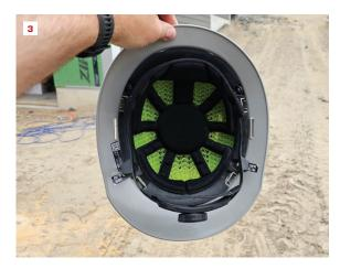
The WaveCel T2+ Max is a Type II hard hat with a wide brim, and top and rear vents for better air circulation (1). Rails for ear muffs and other accessories are incorporated in the design (2). Fit can be adjusted with the oversized dial (3).
