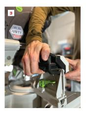
The Reekon M1 is designed to clamp to a miter saw's fence and accurately measure the material being cut (1). The display is large and clear (2), and the spring-loaded clamp provides a strong connection to the fence (3).
