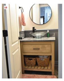
The author tacked the shelf slats to the bottom rails (9), then secured them with pocket screws driven up through the rails (10). The author used a beading bit (11) to shape the edges of a length of poplar, then ripped the bead detail to size on his table saw (12) in order to trim the edges of vanity's inset drawer front (13).
