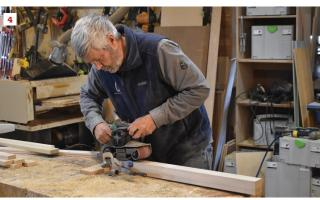
After gluing up poplar blanks for the vanity's corner posts, the author scraped off dried glue (1), then planed the blanks to finish size. The posts have tapered legs, which the author cut with the help of a plywood jig (2, 3). After cutting the tapers in the 2x2 posts, the author used a belt sander to smooth away kerf marks (4).
