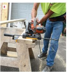
The Skateplate's wide rollers reduce friction and improve accuracy. Rips to the center of a sheet of plywood are possible when a Skateplate is fitted with the optional 10-roller Skateguide with a 34-inch bar (1). The standard four-roller Skateguide with a 17-inch bar comes kitted with the Skateplate combo pack (2).
