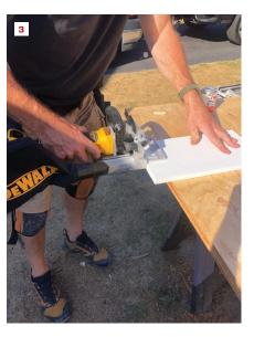
DeWalt's DCW682B cordless biscuit joiner is compatible with all of the company's 20-volt Max batteries (1). The integral fence is easily adjusted without tools for angles between 0 and 90 degrees (2). The tool comes with a dust port and bag (3).
