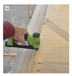
The author used a router to cut 1/4-inch-deep-by-1/2-inch-wide rabbets in the back of the frame to accommodate the 1/4-inch plywood panels (9). When the corners were 90 degrees or greater, he simply clipped the panel corners to fit them into the rabbets (10). To fit the acute angles on the small, triangular corner panels, he used a belt sander to round over the corners (11, 12). The panels are held in place with glue and short wide-crown staples (13).
