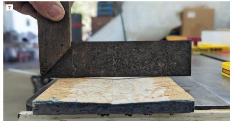
Run one side of the ripped OSB through the saw (5). Then flip the board over and run it through the saw again (6). Feather boards help to hold the board straight and in position. The completed backer board has a recess a little over 1/4 inch deep (7).
