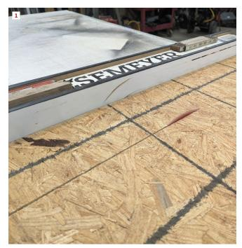
Start by ripping a sheet of  $^{7}$ /1s-inch OSB into  $^{5}$ 1/2-inch widths (1). Set the fence to  $^{1}$ /2 inch (2) and adjust the height of the saw blade to  $^{2}$ 13/1s inches (3). Next, set the bevel of the table saw to 3 degrees. It is important that the blade is tilting toward the fence. If everything is set correctly, the table saw should look like this (4).
