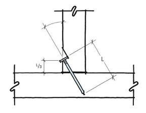
Proper toenailing. When toenailing, place the nail away from the end of the board at a distance that's equal to one-third the length of the nail. With a 2 1/2-inch nail (such as an 8d sinker), start 7/8 to 3/4 inch up from the end and drive it at around a 45-degree angle to exit the center of the stud section. A longer nail (as shown above) would be driven at a steeper angle to exit the center of the stud.
