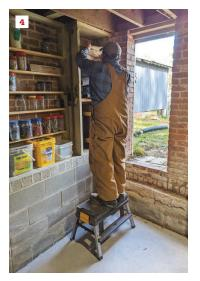
DeWalt's DWST25090 storage step stool consists of a large tool tote and separate step stool that can be clamped together for transport (1). The author uses the stool as a small work platform (2), while the tote stores his cordless tools (3). The stool has a 300-pound load capacity (4).
