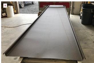
shop. There, I mocked up a  $3^{1/4}$ -inch-by-10-foot piece of drip edge to be sure it would work before making the rest. My guys then took 10-foot sections and slit the necessary stretch-out (a term for the width of metal needed) and started forming the radius drip edge.
