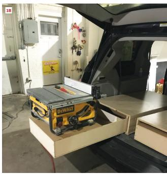
By removing the table saw and placing a piece of plywood over the top, the author can create a track-saw station (15) or large assembly table. Bora's Centipede expanding table offers a useful worktable that sets up quickly (16). For a small work vehicle, the author built rolling drawers—one the width of a miter saw (17) and one the width of a table saw (18)—that can serve as workstations for small jobs.
