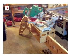
The adjustment bolt for the stock support can also be placed above the rail to hold the support where there isn't a slot (7). The author cut handholds in the saddle box to make it easier to lift the miter saw on and off the Tri-horse rail (8).
