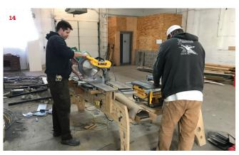
For deck work, the author configures the workstation to support long material (11). When space is tight, the workstation can be configured to take up a small footprint (12). This configuration (13) allows one carpenter to work efficiently. When two carpenters are using the workstation at the same time, the author configures it so they can work comfortably without getting in each other's way (14).
