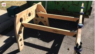
The miter saw table can also be secured to the rail with Trojan Work Center clamps (9). Metal brackets for holding 2x4s clip into the rail holes (10) to create a support table where the author typically places a table saw. The disks on the right-hand rail are rubber-topped Rockler "bench cookies," which clip to the rail to provide an additional work surface.
