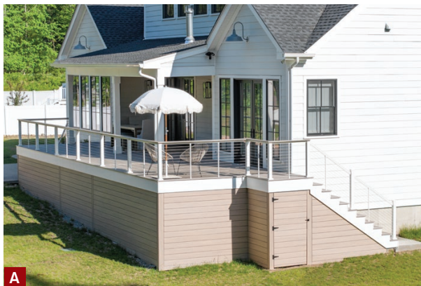
Figure 4. Blocking was also required for the surface-mounted 4x4 rail posts (A). The small landing for the flight of stairs at the end of the deck was conventionally framed and provides access to storage underneath the deck (A). A wider set of stairs at the other end of the deck leads to a poured-concrete patio and sitting area (B).
