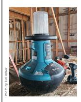
For us, jobsite lighting is a must. In 2005, we invested in the first of a series of plug-in metal halide Wobble Lights, switched to battery-powered lights in 2016, and then graduated to the hugely expensive but really good Milwaukee MX Rocket Tower Light last year. Because we have a lot of Makita XGT tools and batteries, I was interested in trying out the company's 40V XGT LED area light (model ML010G).
