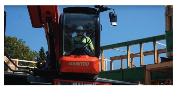
At left, Morton is operating a Manitou MRT 2260 Vision+, one of the two Manitou rotating telehandlers that his company owns. Though he's in the machine's cab here, most of the time he works outside thanks to the this telehandler's remote control functionality.
