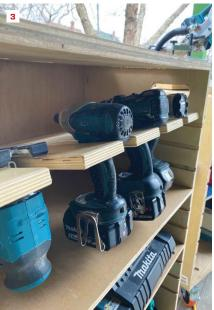
Portable shop. On large trim jobs, the author rolls out tool cases that double as a miter saw stand—a shorter case (1, center) for the saw and taller cases that function as material supports. The cases organize tools by category: pneumatic tools like air guns and a compressor (1, at left); cordless tools and chargers (1, at right); and corded tools in a case with an attached outlet hub (2). Angled tool holders in each case make tools easy to grab but secure for transport (3).
