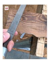
Using an AccuScribe Pro, the author draws the contours of the stone onto the workpiece. Be sure to hold the workpiece parallel to its intended position (9). Test the fit and repeat as needed. A rasp, sander, or knife can be used after the first cut with a jigsaw. Patience is important; you won't get it right the first time (10-12).
