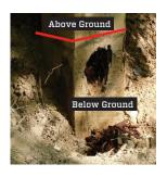
A 10-year-old embedded post treated to the level of UC4A has prematurely decayed where the wood is below ground.
