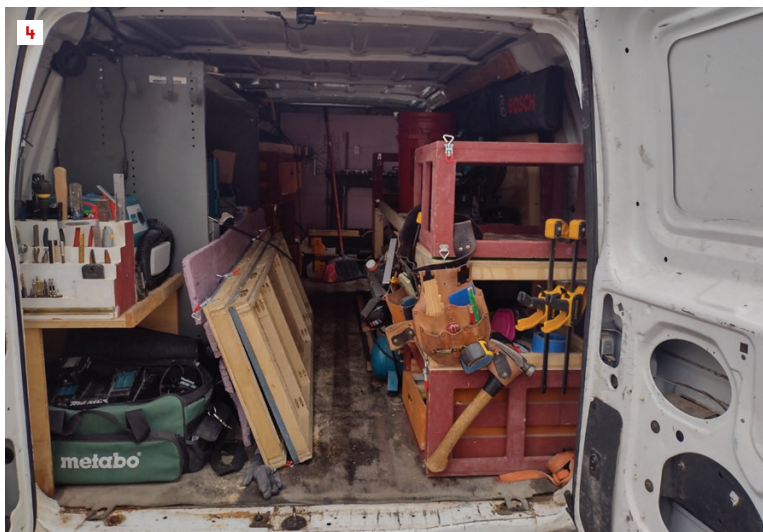
The holdowns on the boxes enable clamping them together as a unit for secure stacking in the author’s van (4). The worktops provide a flat work surface for many tasks. Note the drilled holes for clamps as well as the clips on the edges for hanging tools within easy reach (5).
