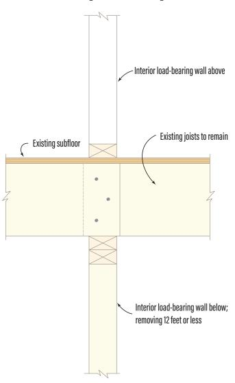
Existing situation. This section drawing shows a bearing wall to be removed to open up space. The illustrations on pages 43 and 44 show different conditions that dictate whether this job could be handled by a competent builder alone or should include an engineer's input.
